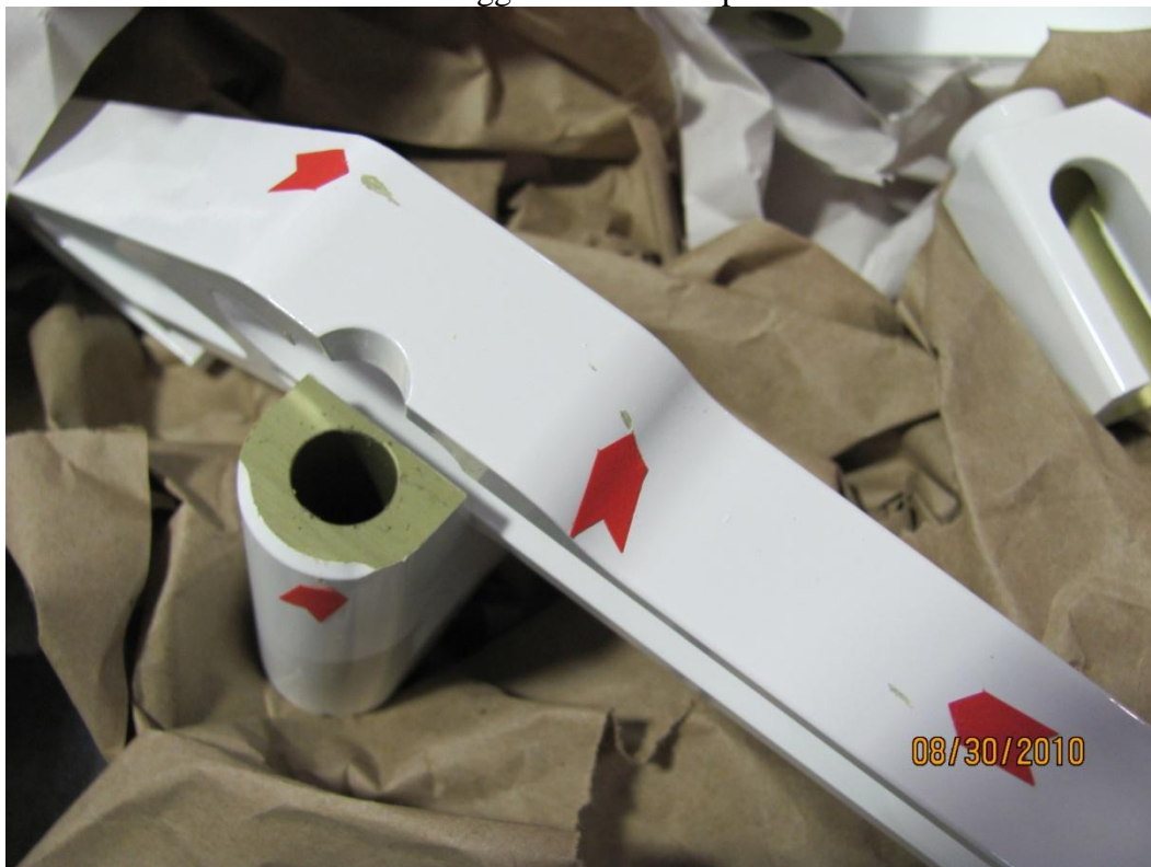
Improper packaging resulting in dings and nicks in paint.
