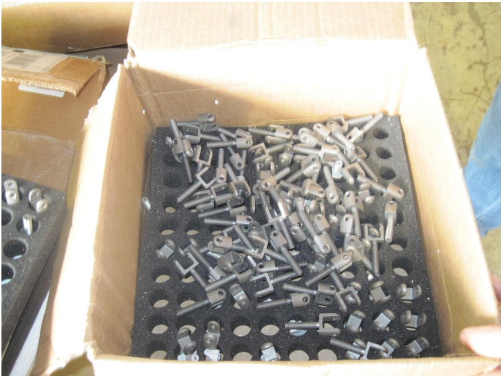
Inadequate, /no-horizontal dividers between foam resulting in damaged parts
