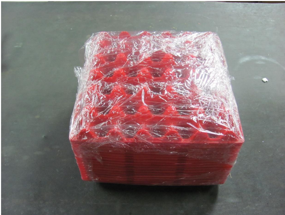
Egg crates properly wrapped to retain parts.
