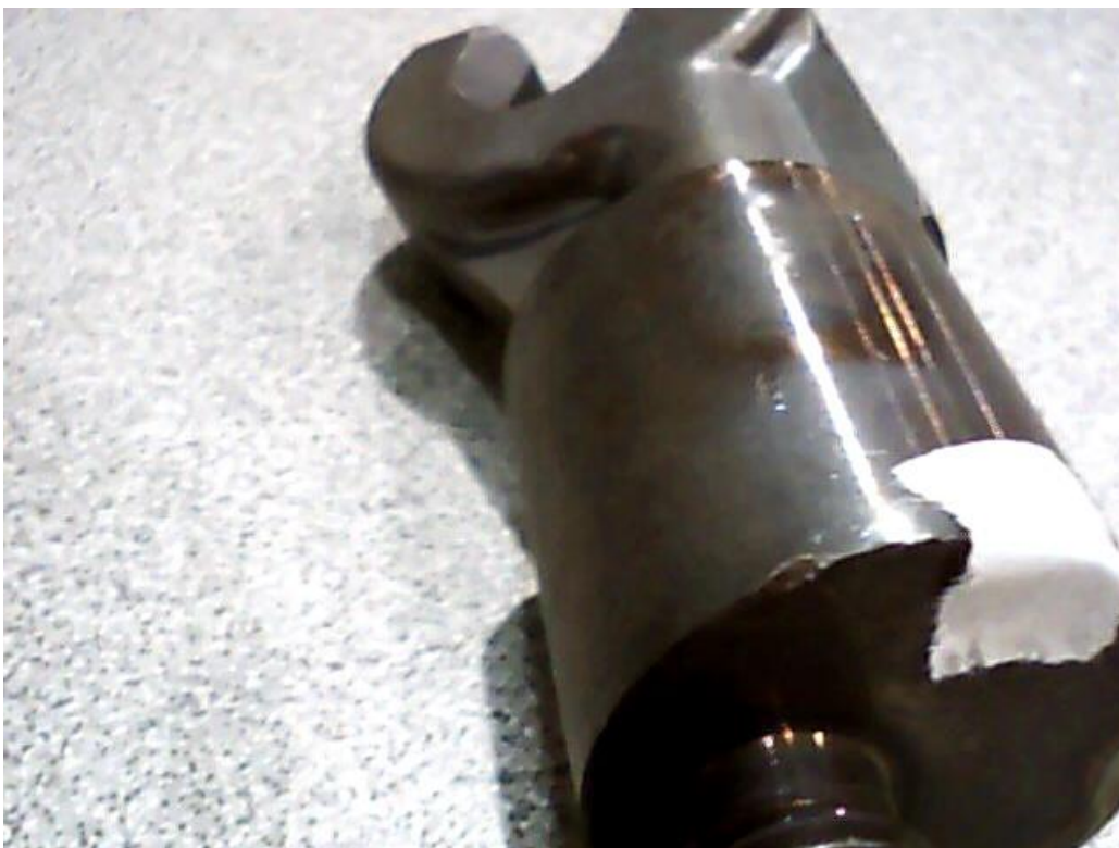
An improperly packaged locking-head – nicks & dings.
