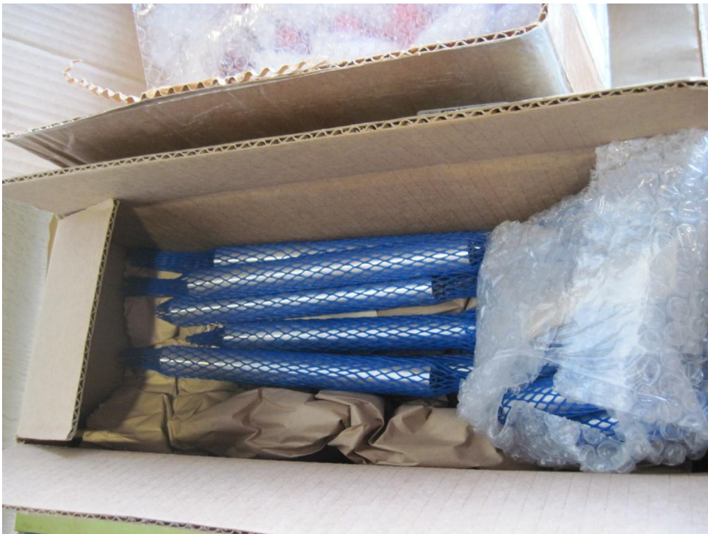
Inadequate tube protection and boxing
