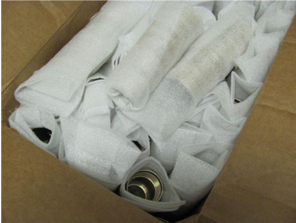
Over-pack Boxes without dividers resulting in damaged parts.
